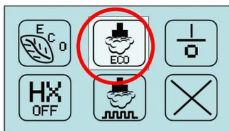
If the steam (service) boiler is set to 127 **and in the advanced menu, "Economy DT" is set to 67**, with an Economy time ("Time Economy" value) of 4. After 4 minutes of inactivity, the steam boiler temperature will reduce to 60C.
