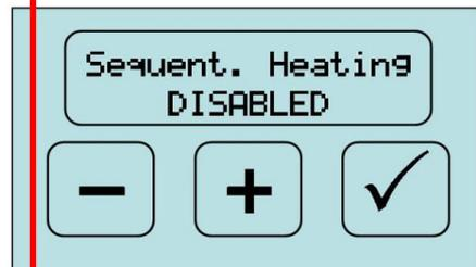
Both boilers heat at once or brew boiler priority, if enabled. Reduces max power consumption to 1500W approx
