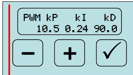
Pump PID settings for controlling pressure, **recommend using these revised values until factory settings are updated**
