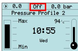
If the steam boiler is switched off in the ECO menu, the display will show "Off" instead of steam temperature.
