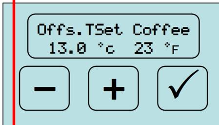
Allows for the drop in temperature of water as it passes from the brew boiler to the coffee. E.g. Brew Boiler water at 107 c, but 94 c is displayed
