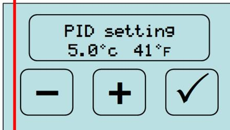
Temperature range around set point where PID operates. We want a larger range for the brew boiler. Your machine may be set to 7C, I recommend you change this to 5C
