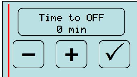
How many minutes (max 999) after machine enters economy mode, before it switches to standby(if not used). **0 to disable**
