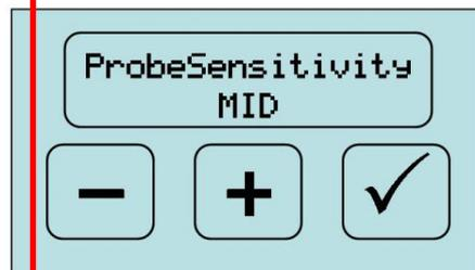
Service boiler autofill probe.. affects fill level, **leave on Mid**. Low allows higher boiler water level, High is less
