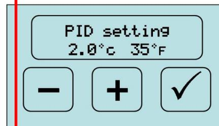
Temperature range around set point where PID operates. We want only a small range for service boiler
