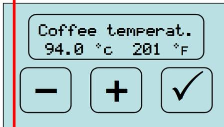
Set the temperature of the brew boiler (also accessible from main menu). I personally use 93C or 94 most of the time.
