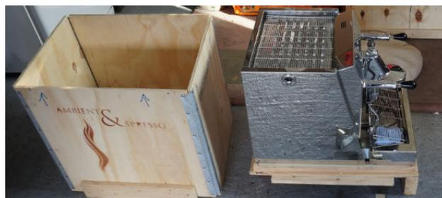
The Vesuvius is secured to the base using rubber transit feet with bolts on the bottom that protrude through the case and are secured with 4 wing nuts, these must be undone. .
