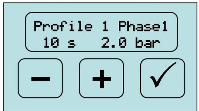
This screen tells us that for the 1st phase (of the 7 phases available), the Vesuvius will deliver a pressure of 2.0 bar for 10s. A global Pump acceleration parameter (page 20) affects how quickly the pump responds and will affect the speed at which any programmed pressure is reached.
