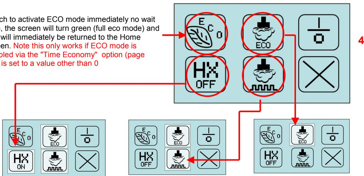
**Brew water preheat, enabled/disabled.** If using high steam temperatures above 127C, **OFF** prevents any possibility of brew water overheating. **Highlighted when ON**
