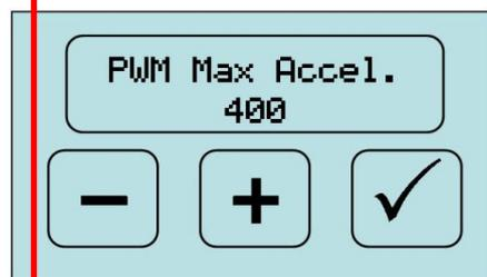
Pump acceleration, speed of response to change. Values above 700 have no effect. **Changing value may require change to pump PID settings**
