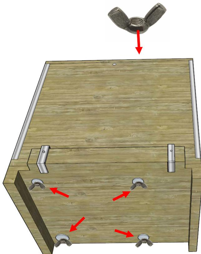
Once the wing nuts have been undone, the Vesuvius will lift away from the base and have 4 soft rubber transit feet attached. These should be removed.
