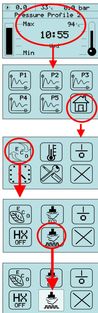
Steam is switched on when the steam button is touched and highlighted, as shown above
