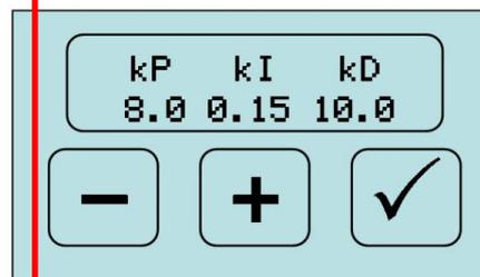
PID settings for steam boiler
