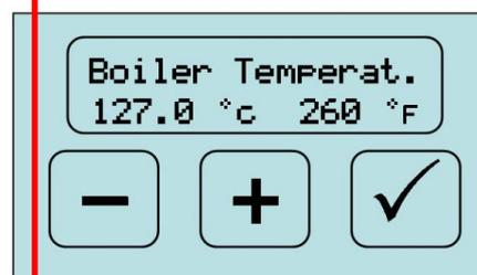
Service (steam) boiler temperature. **I recommend a setting of 127 or 128 (factory use 130)**
